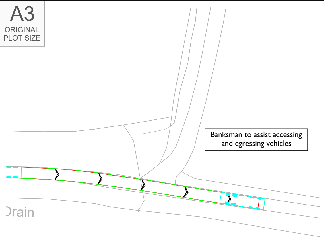
Tipper Vehicle Entering Site
